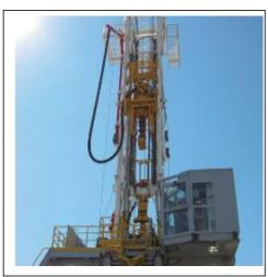
Construction: Consisted of inner rubber layer or stainless steel armoured pipe, reinforced layer of carbon fiber, medium rubber layer, reinforced layer of steel and outer rubber layer of carbon fiber.
